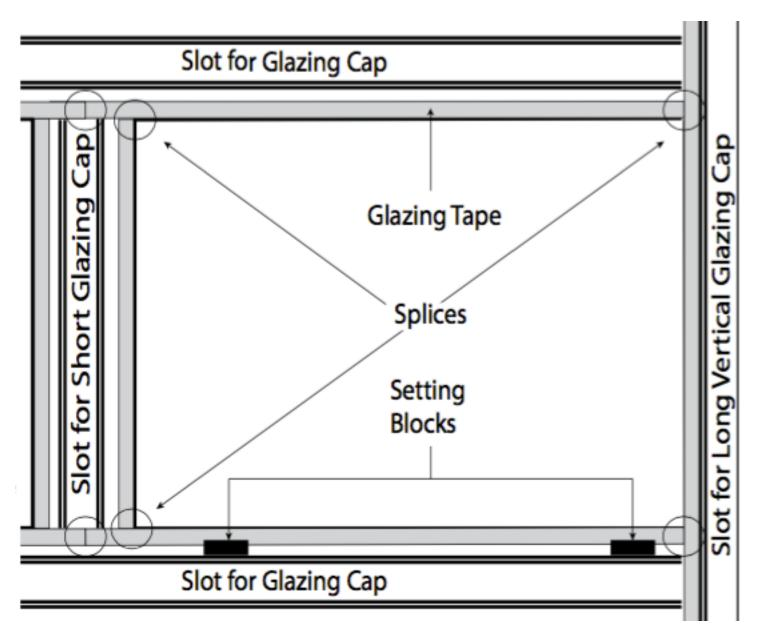
C. Splices in the tape make the glass less likely to stick, so only splice the horizontal strips of tape where the mullions meet the
