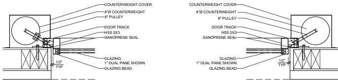
03 DOOR JAMB NON-MOTORIZED SCALE: 1-1/2" = 1'
