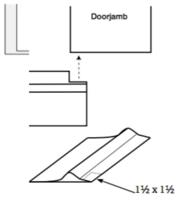
D. Drill pilot holes in the floor for the screws through each of the predrilled holes in the threshold. Move the threshold, and apply a bead of structural adhesive that is 5/16 of an inch thick between the pilot holes where the threshold will lie.
