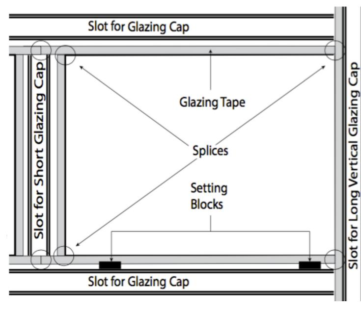
1 Apply the tape and seat the glass panels
