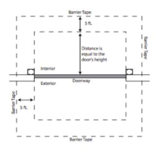
B. Set up a safety zone according to the illustration.
