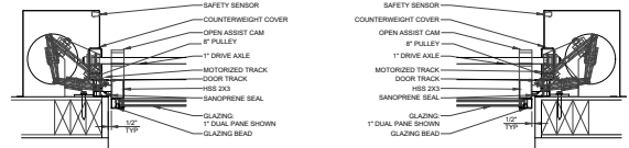
01 DOOR JAMB MOTORIZED SCALE: 1-1/2" = 1'
