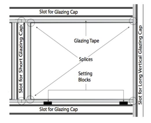
C. Splices in the tape make the glass less likely to stick, so only splice the horizontal strips of tape where the mullions meet the frame and where the vertical cap grooves meet the mullions.
